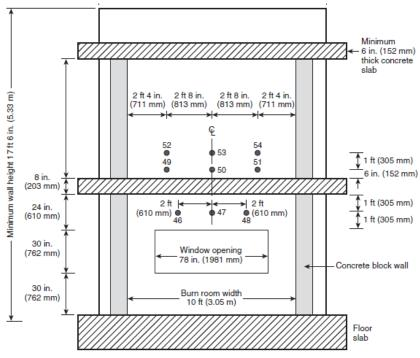
Thermocouples — 1 in. (25 mm) from interior wall surface
